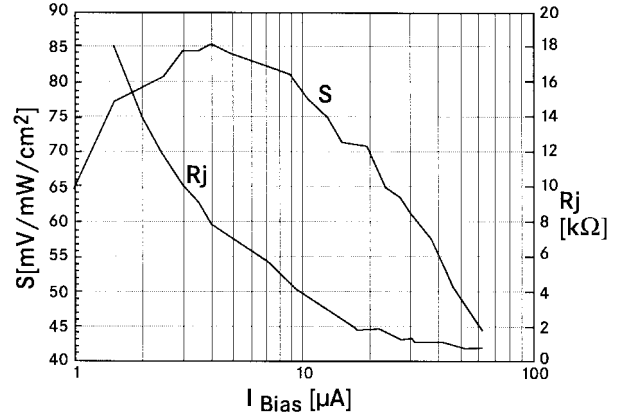
Fig. 10. Sensitivity of the slot-line rectenna and junction resistance versus bias current.
